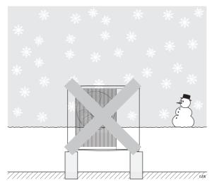
Prevent snow from building up and covering the grilles and drain holes on JÄSPI Inverter Nordic.
