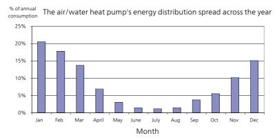
Increasing the indoor temperature one degree increases power consumption by approx. 5%.
